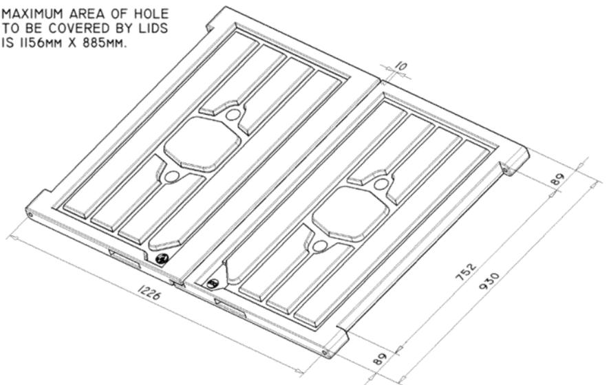
A 10MM GAP BETWEEN LIDS IS RECOMMENDED ON INSTALLATION.
